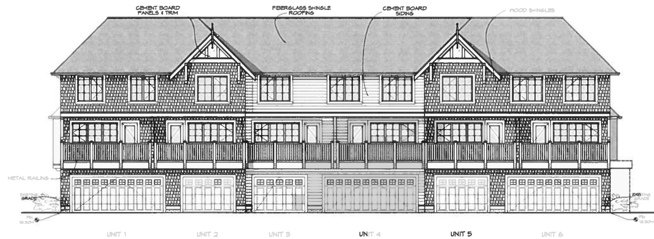
○ Rear Elevation - Building A Scale: 1:100
